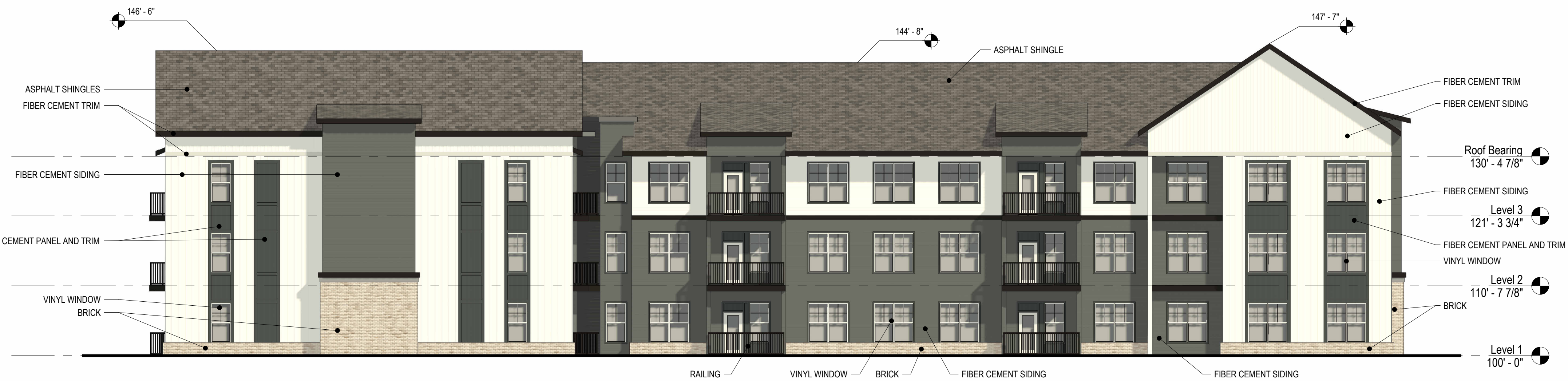
2 BLDG C - WEST ELEVATION A3.4 3/32" = 1'-0"
