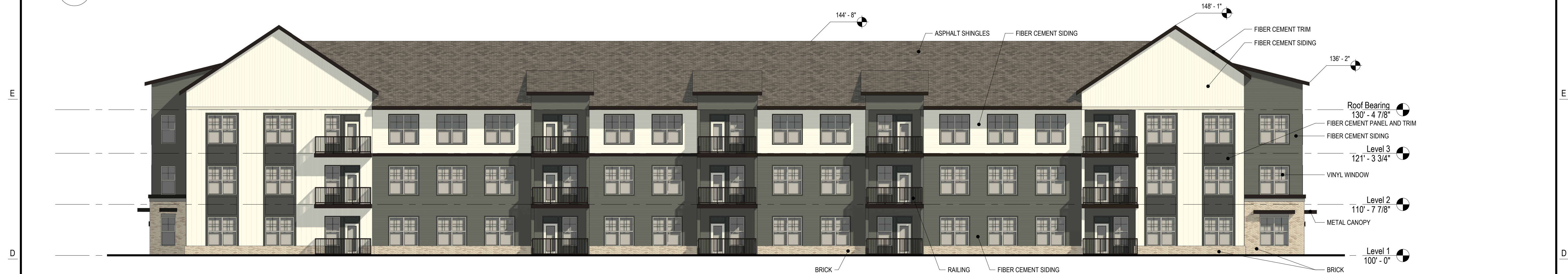
1 BLDG TYPE "B" - FRONT ELEVATION A2.2 3/32" = 1'-0"
